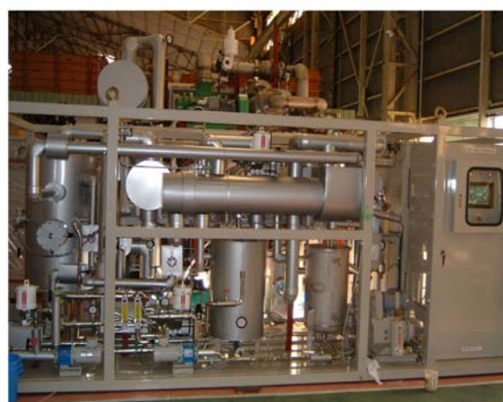
Figure 10. Mitsui demonstration plant in Brazil for the dehydration of bio ethanol by steam permeation using LTA membranes (Ikeda, 2004).
